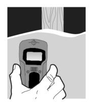
thickness of the detected wall. The calibration is finished when the sound stops. You can process joists detection now and please always press the power button during the detecting course.
